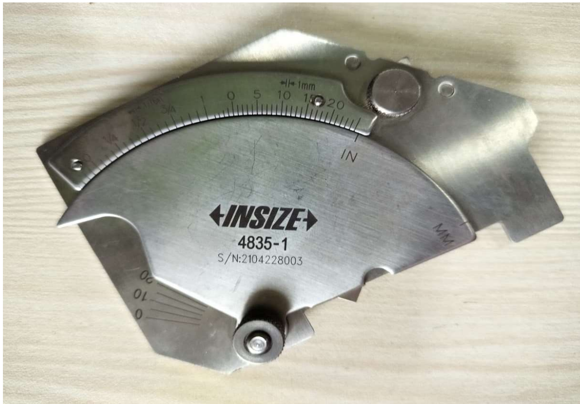
Gauge for checking weld size (I-5.16)
